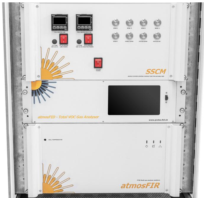
Protea FTIR and FID analysers are combined in full CEM with sampling system control and data reporting.
